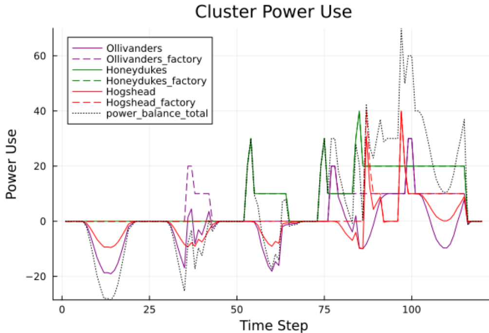
Figure 4.3: Energy profiles of the Cluster case and r = 0.5 . They represent the energy balance of each firm, also showing a profile with only the factory demand without PV as a dashed line, and the total energy balance of all firms in a black, dotted line.
