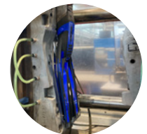
Snorkelling fin as the product of an injection moulding machine at SEAC
